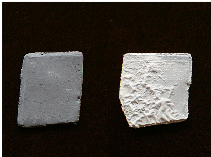
Fig. 2. Lead sensors with alteration products of gray (left) and white color (right).
