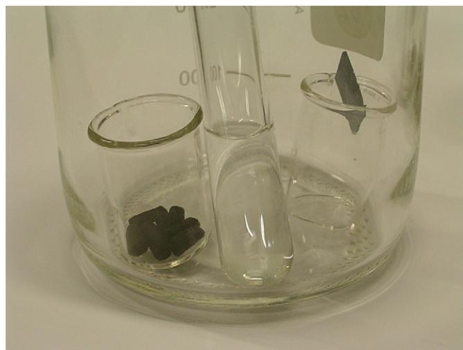
Fig. 1. Experimental setup: goblet with adsorbent (left), test tube with the acetic acid solution (center), and lead sensor at the top of a goblet (right).
